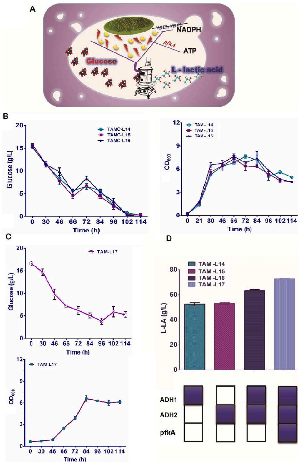
**Fig. 5.** Regulation of energy and redox cofactor compensation to promote L-LA bioproduction. (A) Schematic diagram of L-LA bioproduction regulated by energy and REDOX factors. (B) OD<sub>600</sub> values and glucose consumption of strains TAM-L14 (TAM-L13ΔNDE1), TAM-L15 (TAM-L13ΔNDE2), and TAM-L16 (TAM-L13ΔNDE1ΔNDE2). (C) OD<sub>600</sub> values and glucose consumption of strain TAM-L17 (TAM-L16::*pfkA*). (D) L-LA bioproduction results of strains TAM-L14–TAM-L17.
